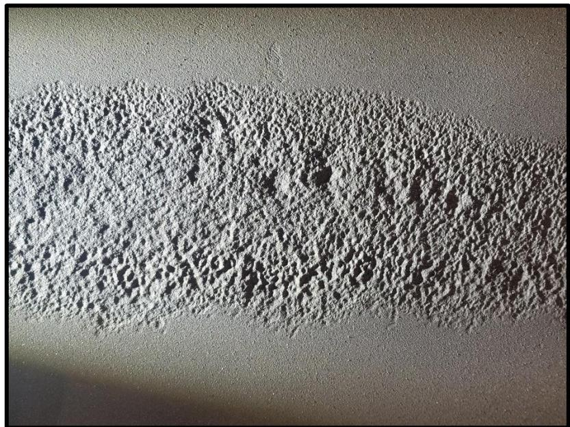
Typical of many of the contact points showing corrosion pitting.
