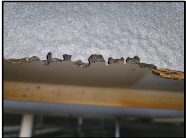
Post-blast outer rafter (worst side of tank).
