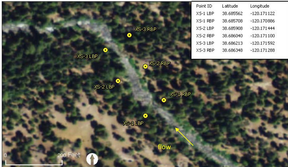
Figure 3-1. Site map of Forgotten Flat site showing cross-section endpoints and coordinates (in decimal degrees). LBP is left bank pin and RBP is right bank pin.
