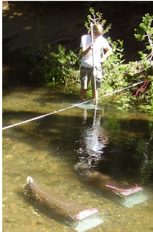
Figure 4-2 Helly-Smith bedload samplers (right) and sampling with Helly-Smith along a cross-section (left)
