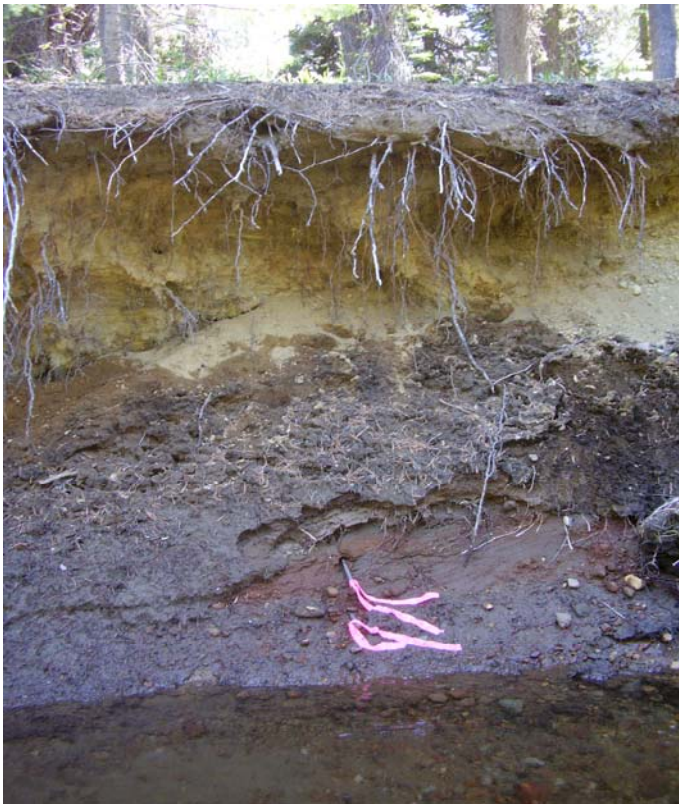
.26 ft bank retreat at Pin 3 and .13 ft at Pin 2 after 24 cfs flow release
