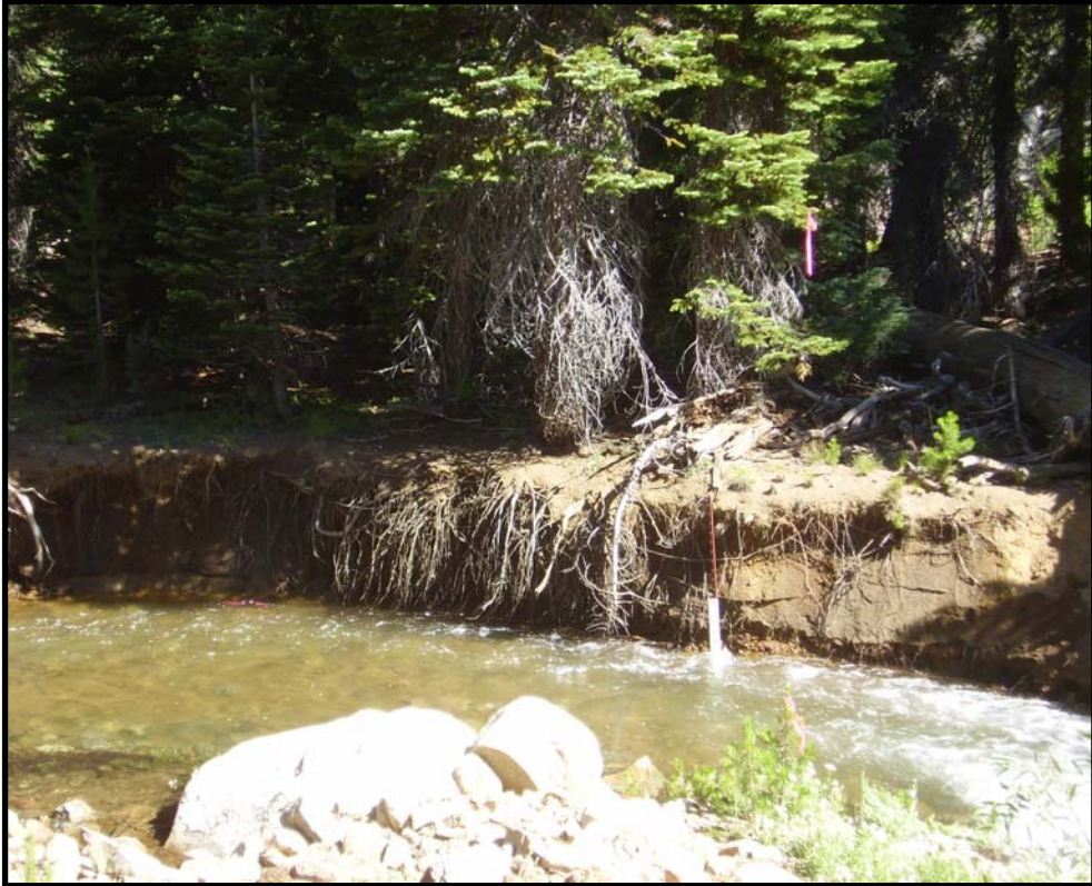
Right bank above large woody debris jam, staff gage 3 at 9.5 cfs (top) and 24 cfs (bottom)
