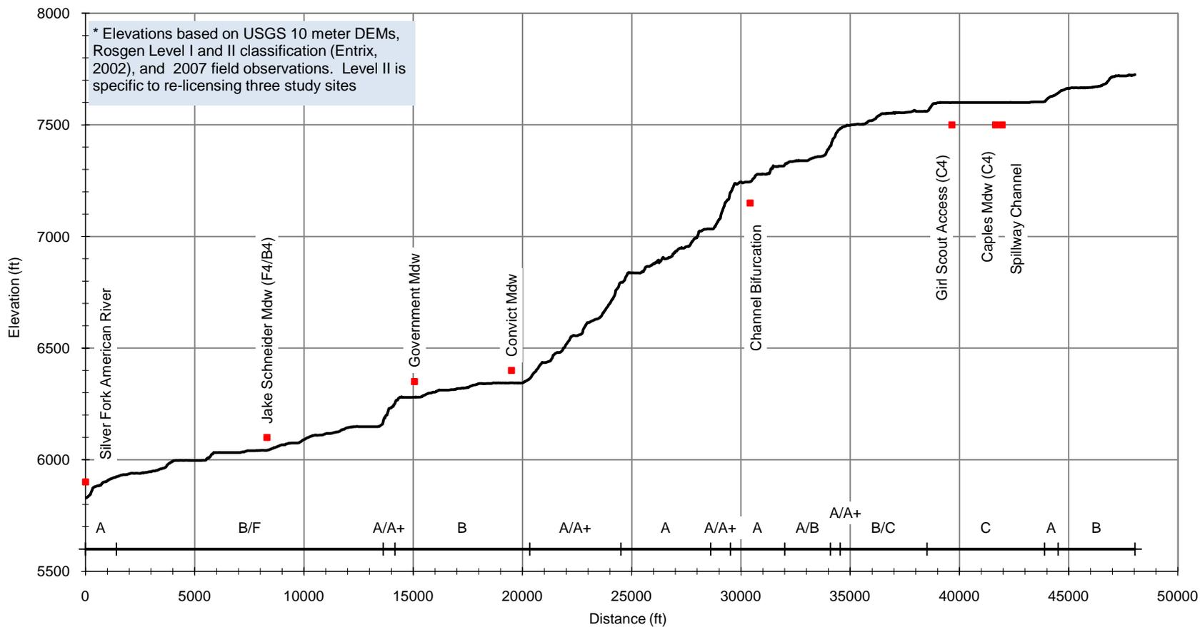
Figure 2-3 Caples Creek Channel Elevation Profile and Rosgen Level I and II Classification
