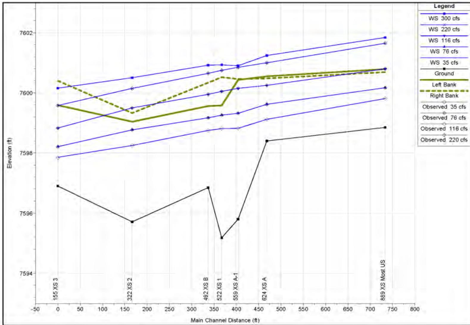
Figure 4-3 Thalweg, left and right top of banks, modeled water surface elevation at Caples Meadow Study Site
