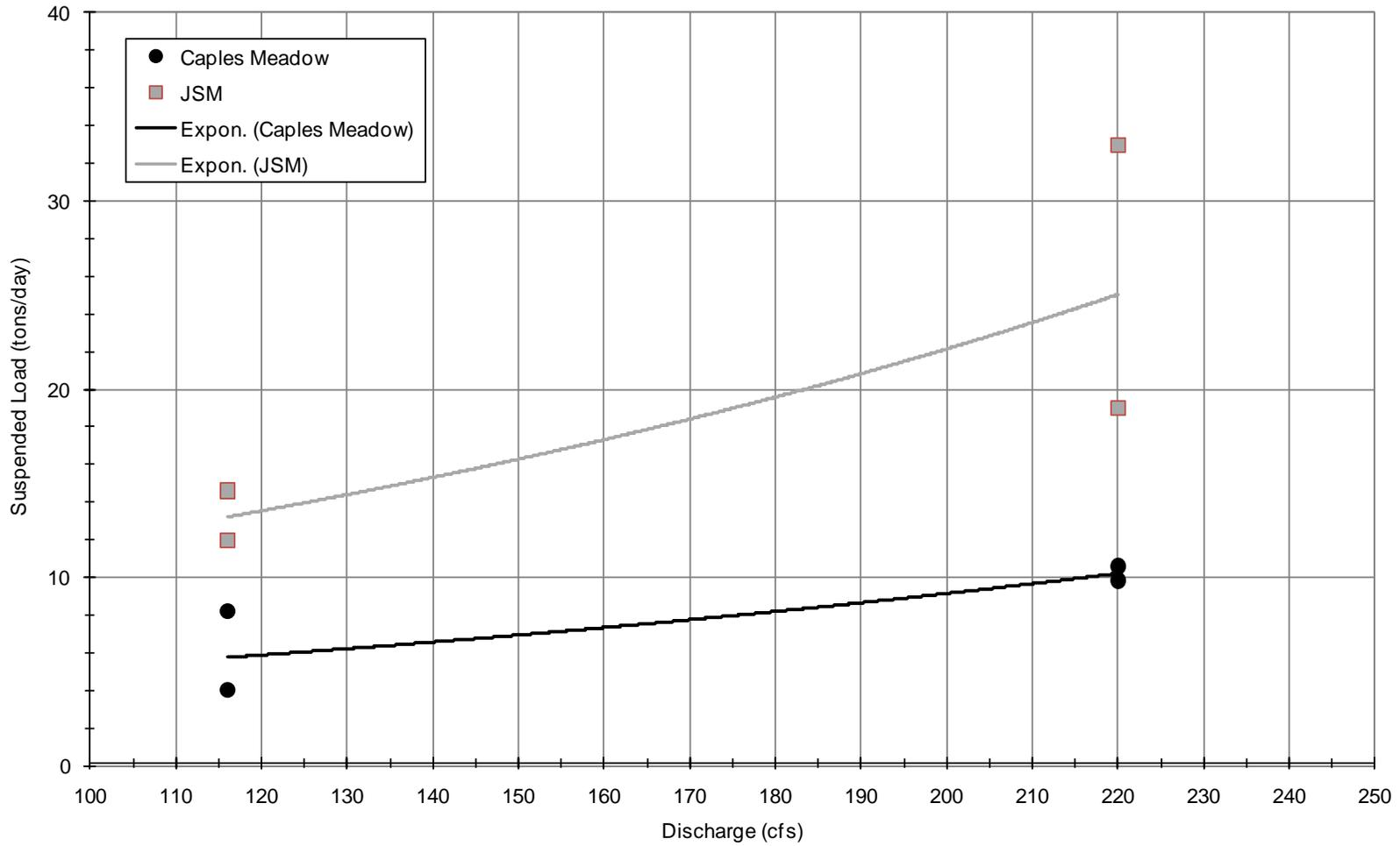
Figure 3-1 Suspended Sediment Load Transport Rates Measured at Caples Meadow and Jake Schneider Meadow
