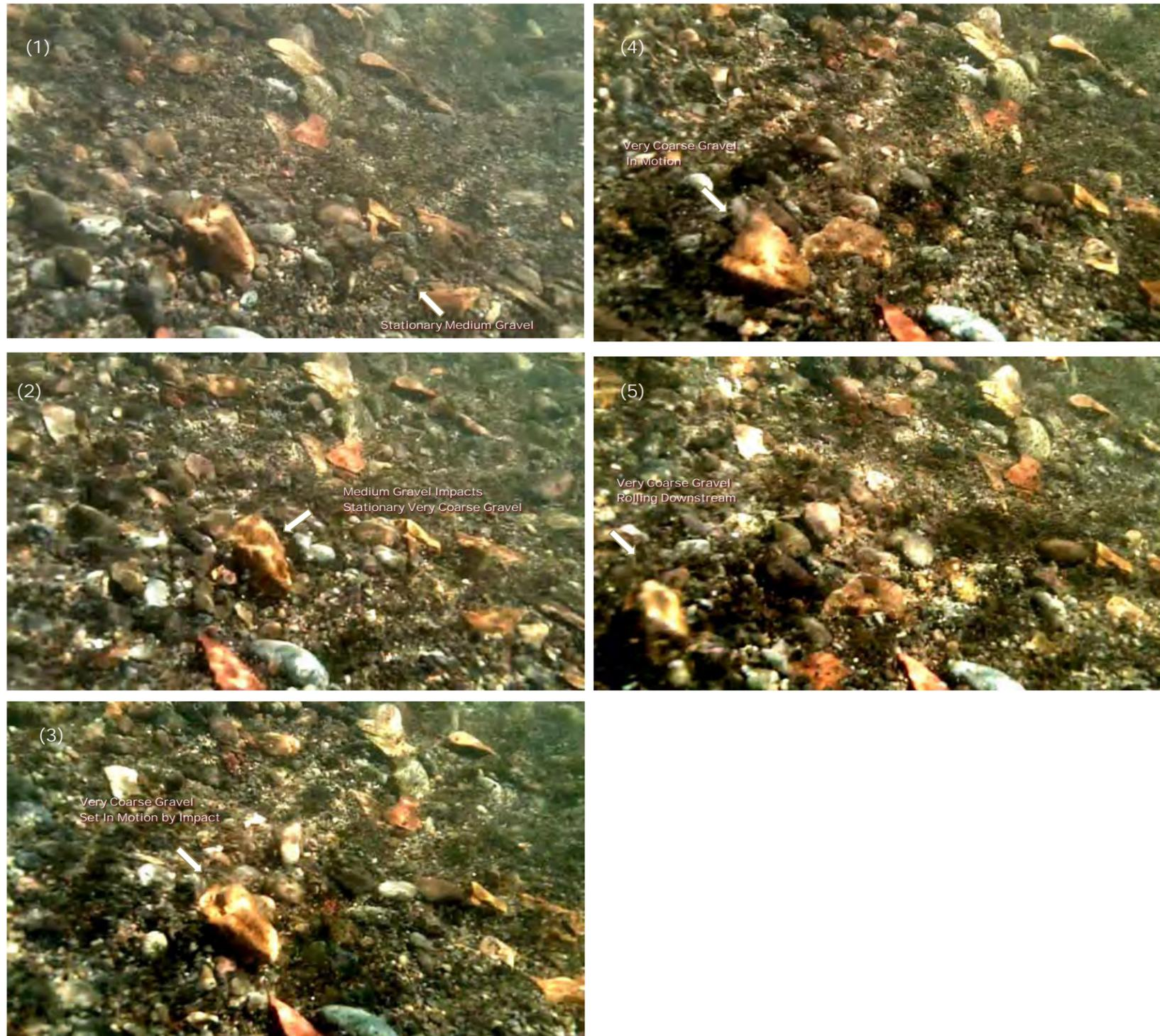
Photo 3-1 Still frames from video taken downstream of Caples Meadow XS 3 on August 5, 2010 at approximately 220 cfs. The photo sequence shows bedload movement
