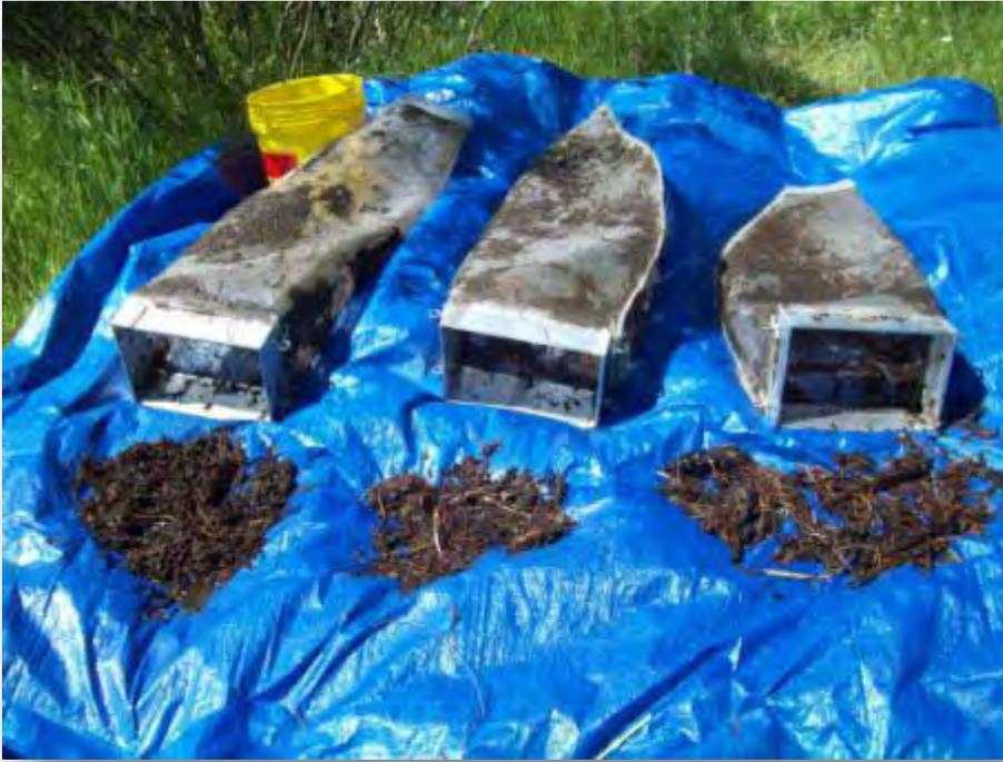
Photo 3-3 Organic debris from the bedload traps deployed at Caples Meadow XS A
