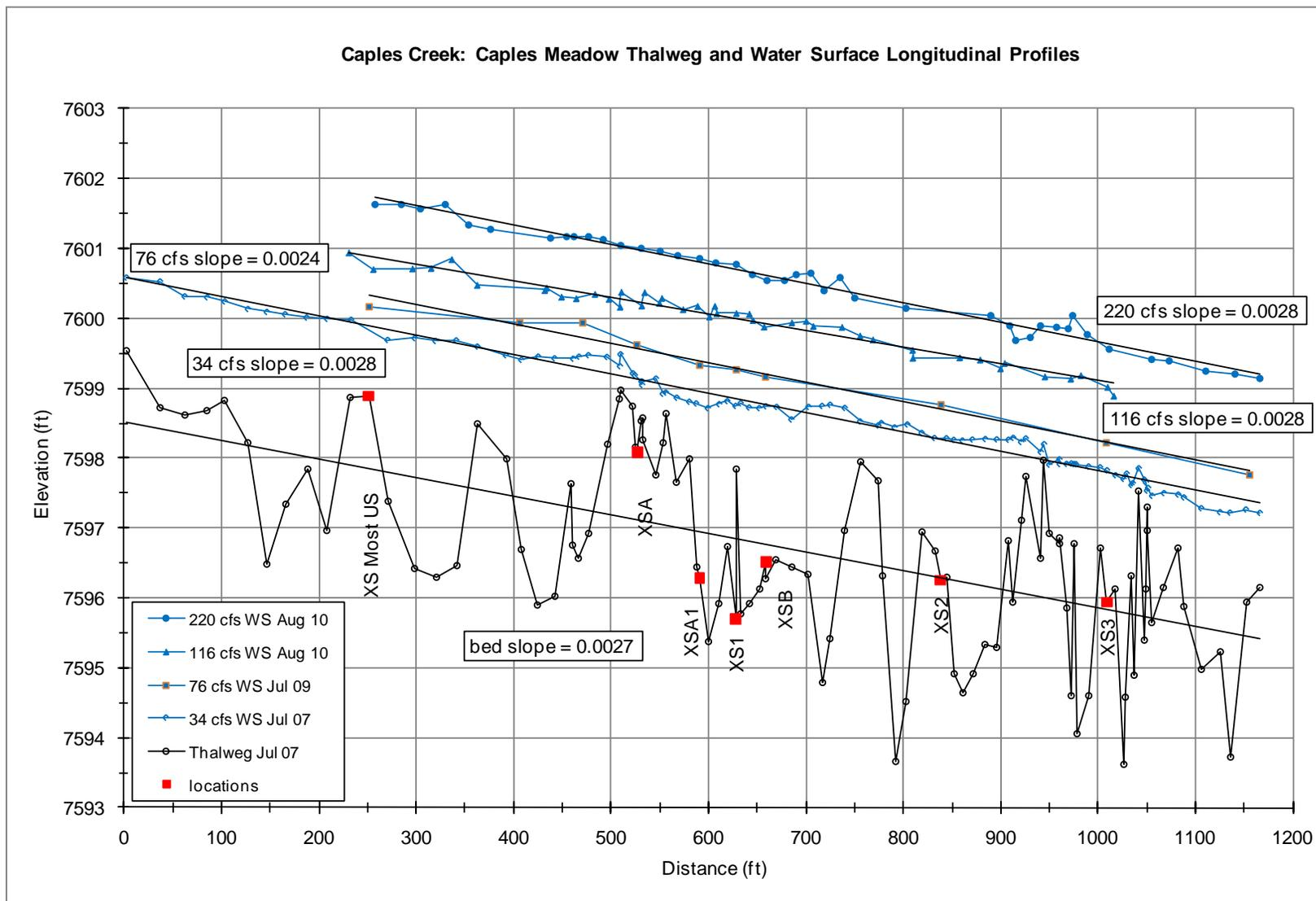
Figure 4-1 Surveied Water Surface and Thalweg Elevation Profiles at Caples Meadow for Calibration Flows
