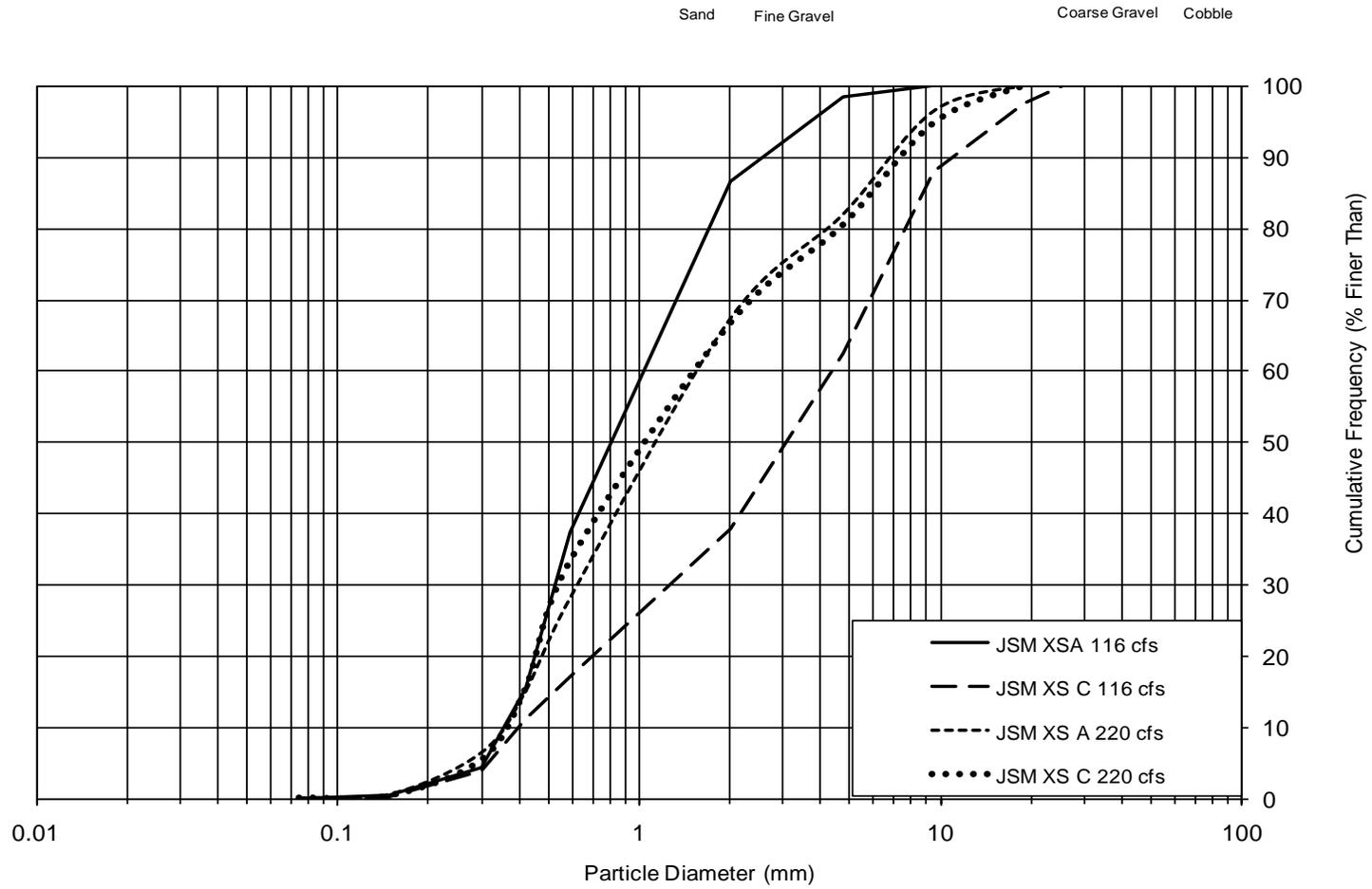
Figure 3-5 Bedload Grain Size Distributions Measured with Helley-Smith Sampler at Jake Schneider Meadow
