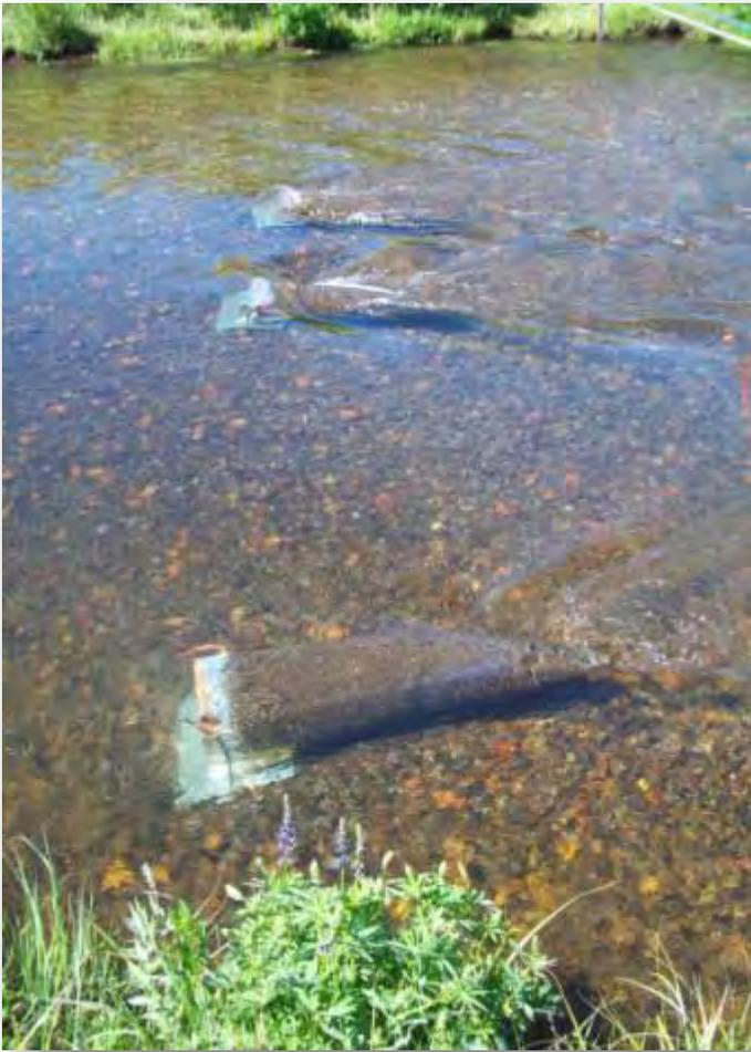
Photo 3-2 Bedload traps deployed at Caples Meadow XS A prior to the 116 cfs test flow
