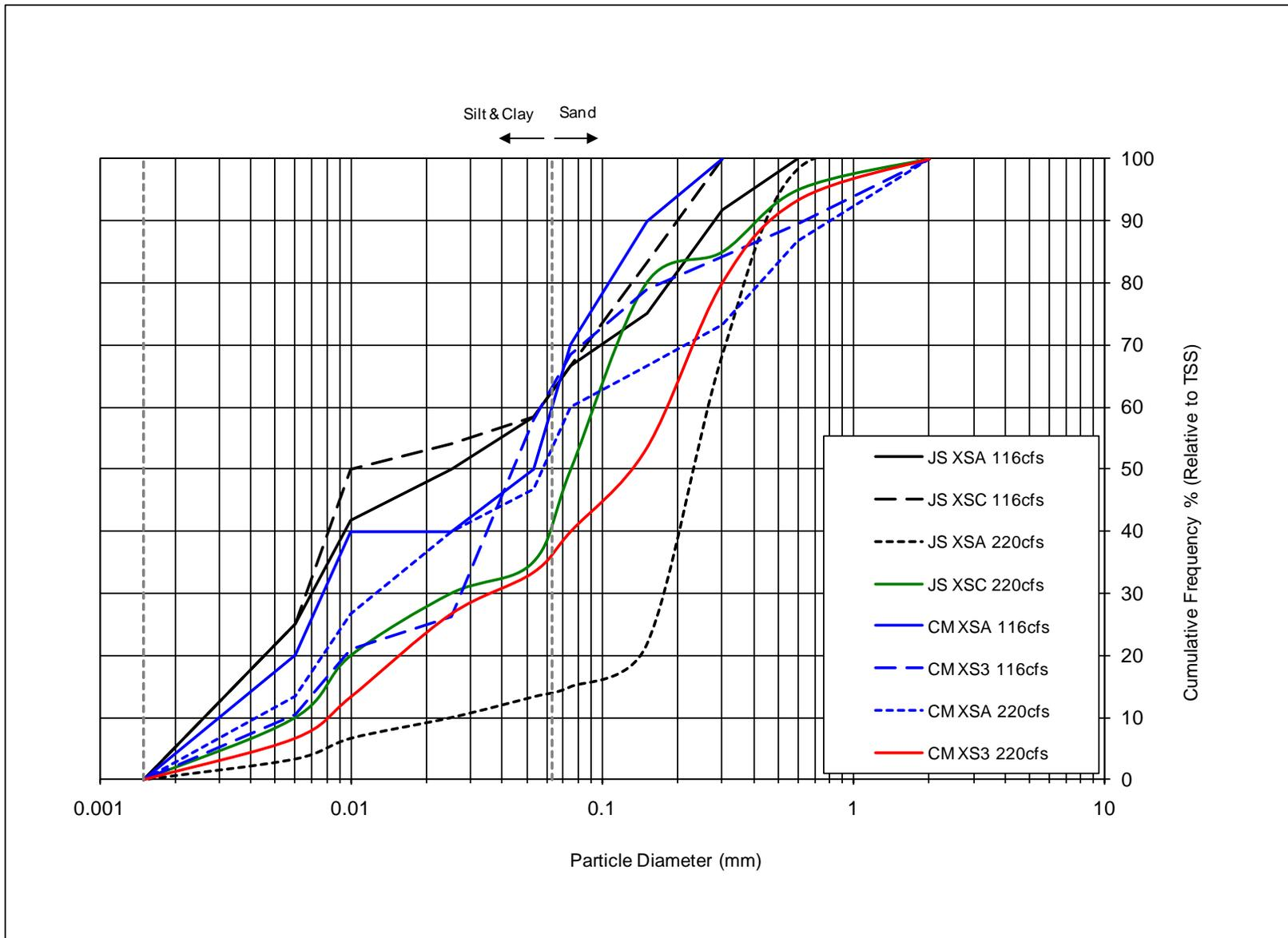
Figure 3-2      Suspended Sediment Grain Size Distributions Measured at Caples Meadow and Jake Schneider Meadow
