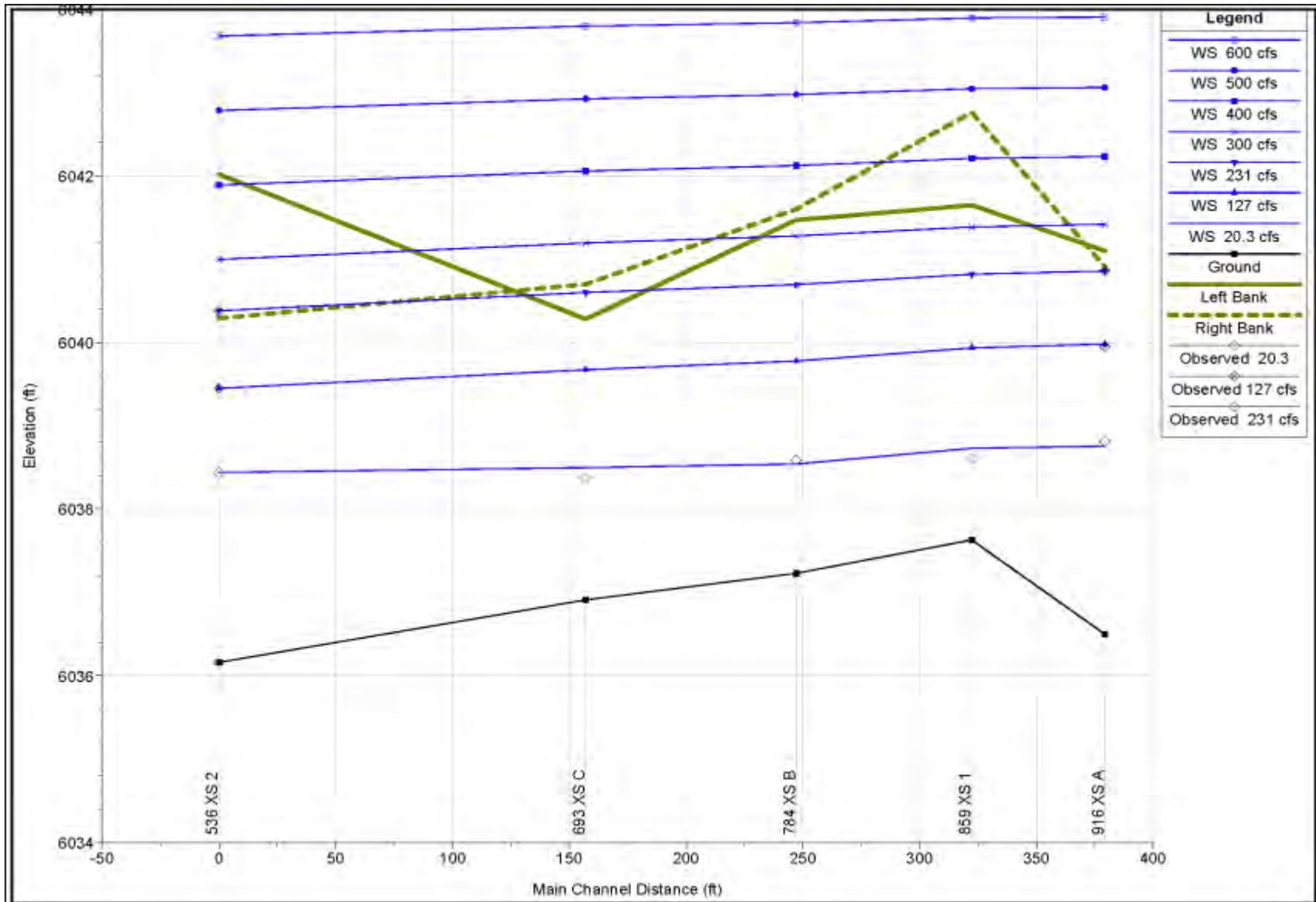
Figure 4-4 Thalweg, left and right top of banks, and modeled water surface elevation at JSM Study Site
