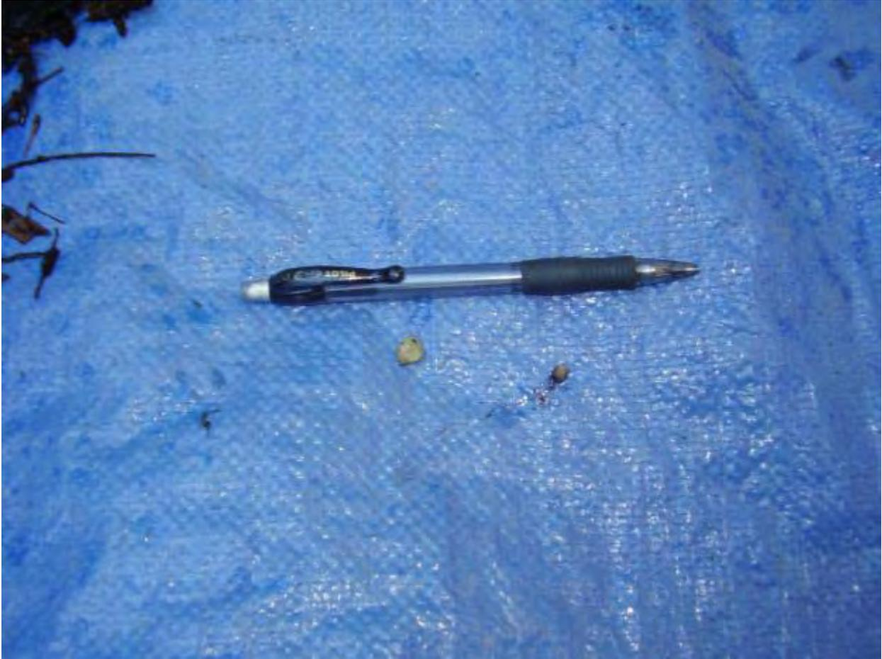
Photo 3-4 Fine Gravels Caught In Net Frame Sampler during 116 cfs Flow at JSM
