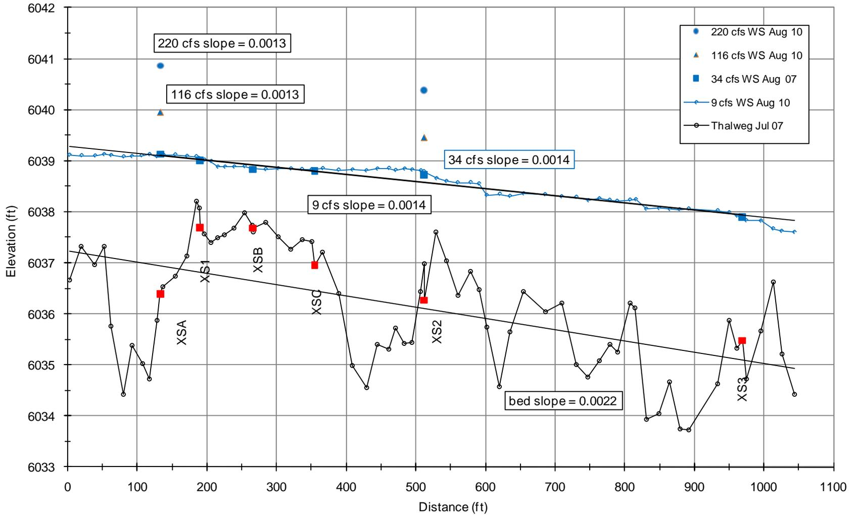
Figure 4-2 Surveyed Water Surface and Thalweg Elevation Profiles at JSM for Calibration Flows
