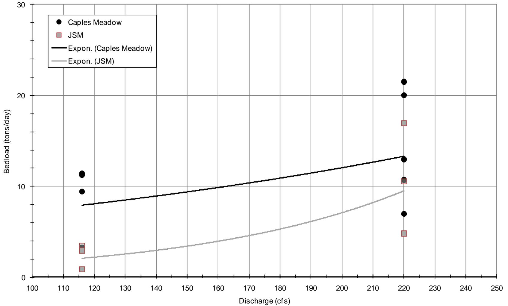
Figure 3-3 Bedload Transport Rates Measured with Helley-Smith Sampler at Caples Meadow and Jake Schneider Meadow
