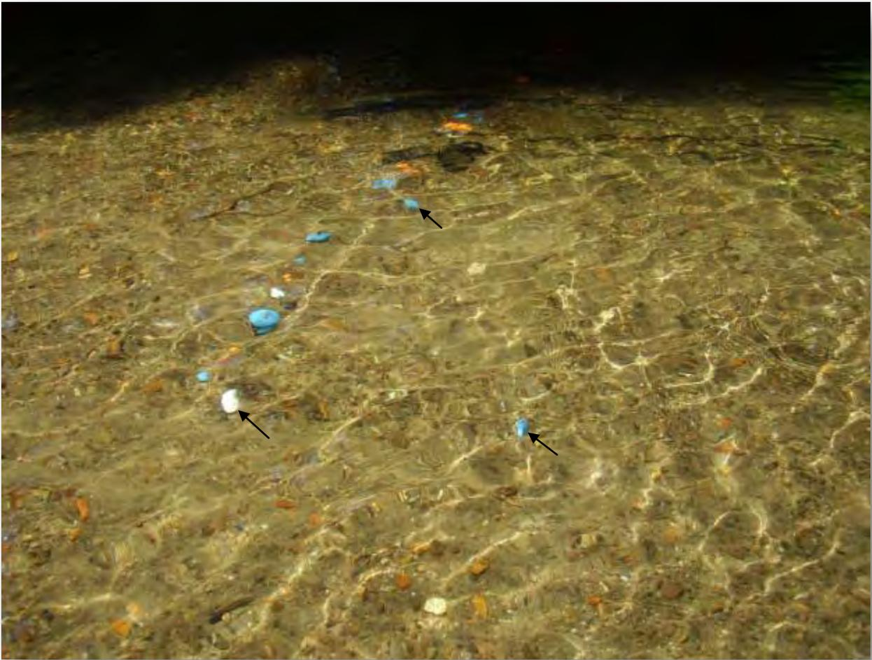
Photo 3-5 Tracers at JSM XS-C After 220 cfs Flow. Three tracers that moved are marked with arrows
