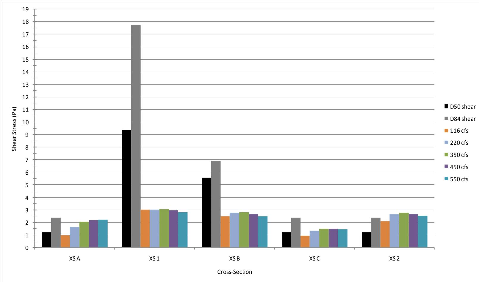
Figure 4-5 Modeled shear stresses compared to the shear stress needed to mobilize the  $D_{50}$  and  $D_{84}$  at Jake Schneider Meadow
