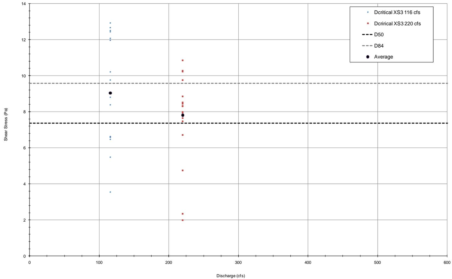
Note: Bed shear stress data points that plot above the horizontal lines indicate the shear stress is great enough to mobilize the D<sub>50</sub> or D<sub>84</sub> sediment.
