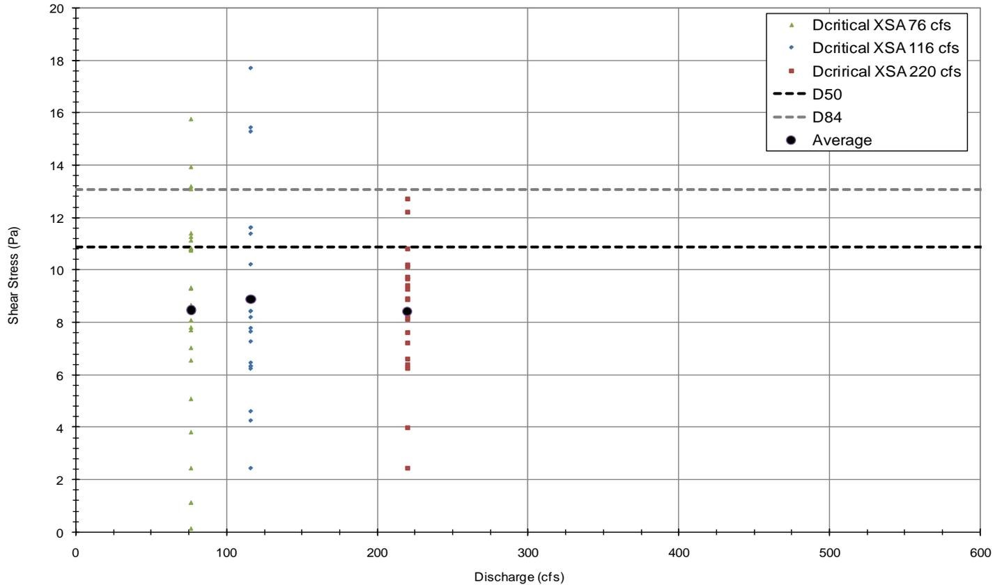
Note: Bed shear stress data points that plot above the horizontal lines indicate the shear stress is great enough to mobilize the D<sub>50</sub> or D<sub>84</sub> sediment
