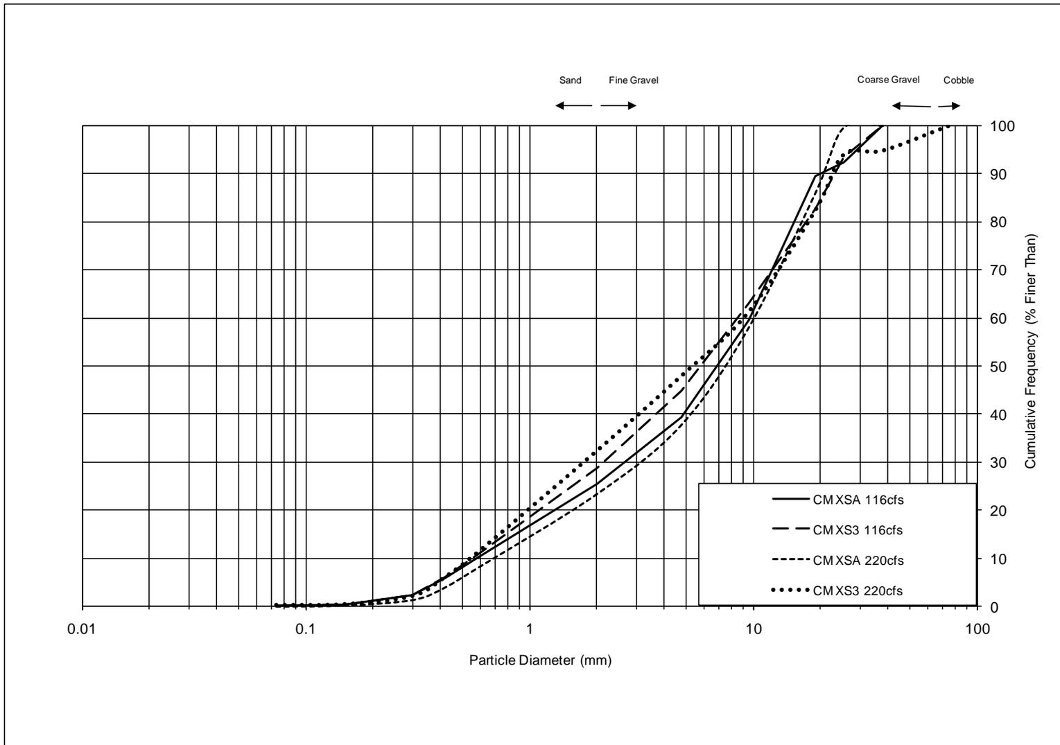
Figure 3-4 Bedload Grain Size Distributions Measured with Helley-Smith Sampler at Caples Meadow
