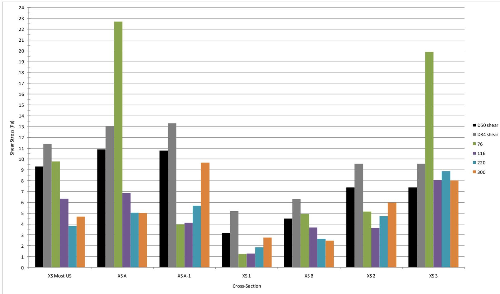
Figure 4-6 Modeled shear stresses compared to the shear stress needed to mobilize the D<sub>50</sub> and D<sub>84</sub> at Caples Meadow Study Site
