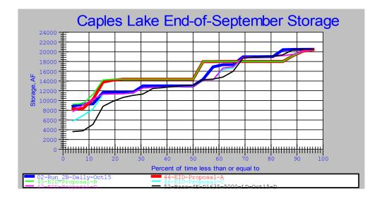
As in August, the different storage targets cause a change in the operation of Caples Lake. In the wettest years, the D1635 storage targets result in higher Caples Lake storage 30% of the time.
