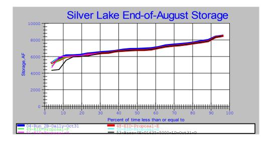
The end of August storage chart shows that the storage is falling due to decreasing inflows, releases to meet minimum flow requirements, leakage, and evaporation.
