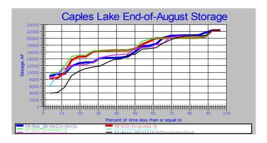
The plot above shows the impacts of the D1635 storage targets versus the Alpine County storage targets. Proposals E and F with the Alpine County storage targets clearly result in higher storage levels in about 70% of the years.
