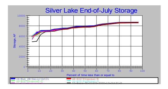
Water is stored through the summer because in accordance with the Silver Lake Agreement. No discretionary releases are made until after Labor Day.
