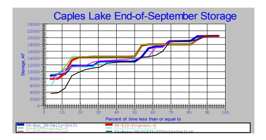
As in August, the different storage targets cause a change in the operation of Caples Lake. In the wettest years, the D1635 storage targets result in higher Caples Lake storage 30% of the time. In other years, Alpine County storage targets result in higher Caples Lake storage.
