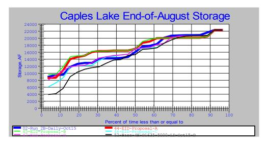
The plot above shows the impacts of the D1635 storage targets versus the Alpine County storage targets. Proposals A and B with the Alpine County storage targets clearly result in higher storage levels in about 70% of the years.
