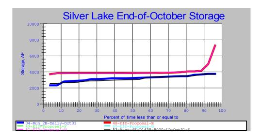
Silver Lake storage at the end of October should be near the DSOD level of 3,756 AF. In most cases the level is at or below 3,756 AF. However, in a few years the basin experienced some late October storms, which pushed the lake level up.
