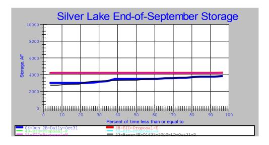
The end of September storage target is 4,200 AF and is attainable in all years for all proposals. The storage is brought down steadily from Labor Day to this point. 4,200 AF is higher than the 3,756 AF required by DSOD on November 1, but provides enough water to ensure minimum flow requirements and consumptive use demands are met while not bringing down the reservoir below 3,756 AF before November 1.
