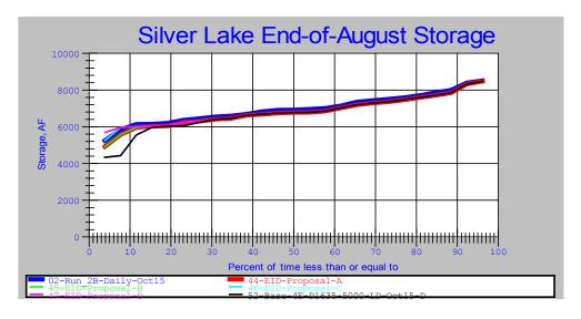
The end of August storage chart shows that the storage is falling due to decreasing inflows, releases to meet minimum flow requirements, leakage, and evaporation.
